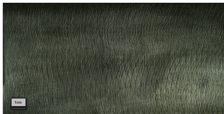
Fig. 3. Weld 2 with a subsurface crack (weld cap removed).
