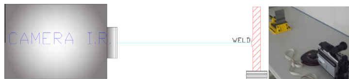
Fig. 5. Cooling monitoring with IRT.
