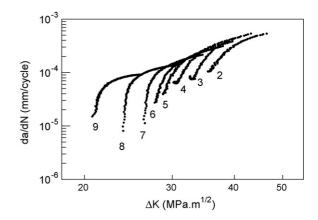
Fig. 9. Fatigue crack growth laws (hot rolled steel E0). The number next to each branch of the curve indicates the fatigue step associated with it.
