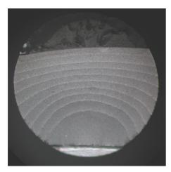
Fig. 6. Fatigue surface (cold drawn steel E7).
