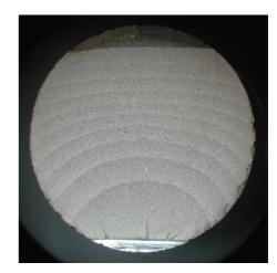
Fig. 5. Fatigue surface (hot rolled steel E0).
