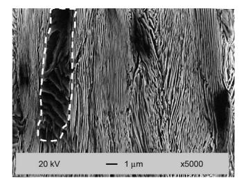
Fig. 13. Pearlitic pseudocolony in the cold drawn wire (in the photograph, the horizontal side is associated with the radial direction in the wire and the vertical side corresponds to the wire axis or cold drawing direction).
