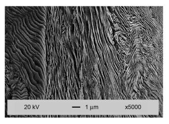
Fig. 12. Longitudinal metallographic section of the cold drawn wire (in the photograph, the horizontal side is associated with the radial direction in the wire and the vertical side corresponds to the wire axis or cold drawing direction).
