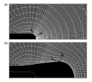
Fig. 16. Initial undeformed mesh at the crack tip (a) and deformed mesh (b) at the unloading phase after fatigue cycles, showing large deformations and rotation of axes from x-y to x'-y'.
