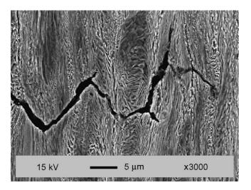
Fig. 15. Metallographic cut showing the fatigue crack growth in the cold drawn wire E7 (crack propagation from left to right).
