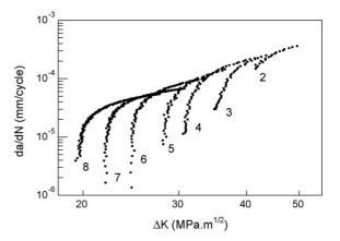
Fig. 10. Fatigue crack growth laws (cold drawn wire E7). The number next to each branch of the curve indicates the fatigue step associated with it.
