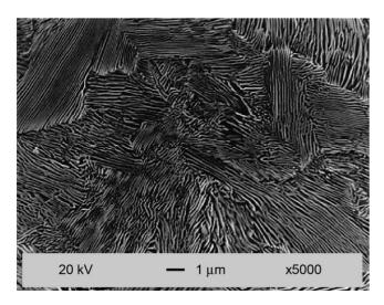
Fig. 11. Longitudinal metallographic section of the hot rolled bar (in the photograph, the horizontal side is associated with the radial direction in the bar and the vertical side corresponds to the bar axis).
