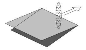
Fig. 18. Scheme showing crack growth by fatigue in mode I after the crack has reached a pearlitic pseudocolony, due to the geometrical constraint produced by the rest of the points of the crack front which therefore tends to propagate in the original direction.
