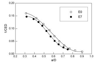
Fig. 4. Dimensionless compliance for both steels.
