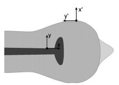
Fig. 17. Scheme showing crack tip blunting and posterior crack growth by fatigue in mode I after the crack has reached a pearlitic pseudocolony.
