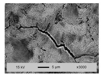
Fig. 14. Metallographic cut showing the fatigue crack growth in the hot rolled bar E0 (crack propagation from left to right).
