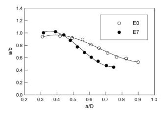
Fig. 8. Evolution of the crack aspect ratio a/b in the hot rolled steel (E0) and the cold drawn wire (E7).
