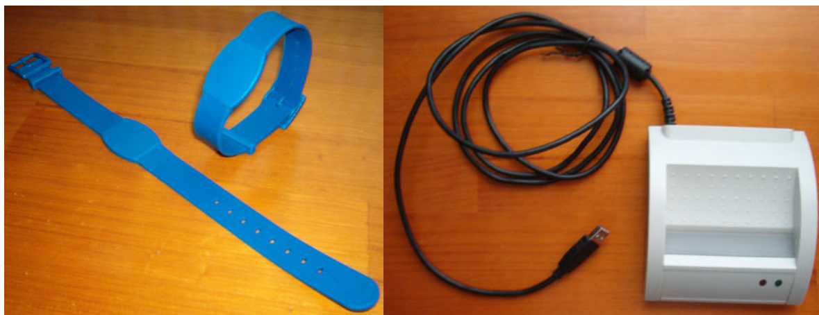
Fig. 2. RFID Technology used in ALZ-MAS: two RFID wrist bands (left); a USB Desktop Reader (right)
