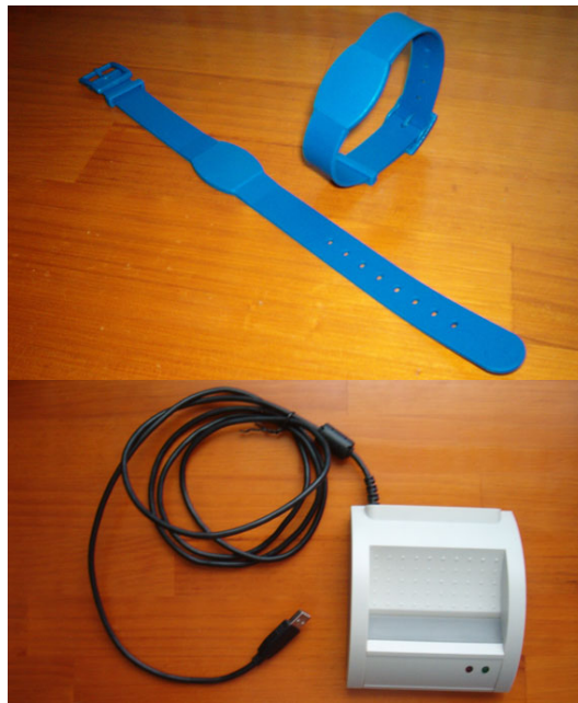
Fig. 4. RFID Technology used in ALZ-MAS: two RFID wrist bands (up); a USB Desktop Reader (down)
