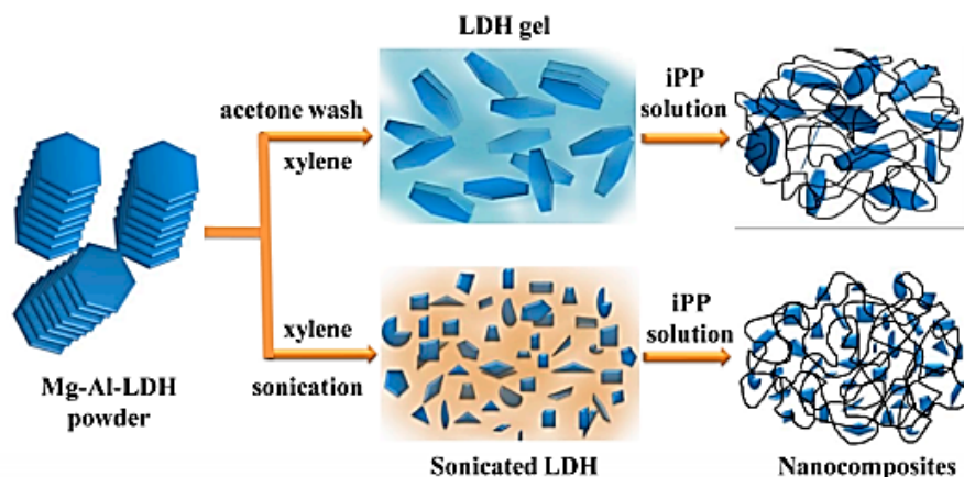
Figure I.20. Preparation of Mg-Al-LDH isotactic polypropylene nanocomposites [237].
