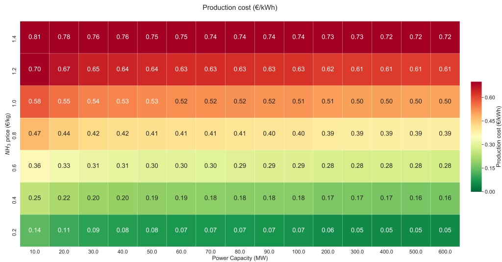
Figure 9: Effect of the ammonia price and the facility capacity in the power production cost
