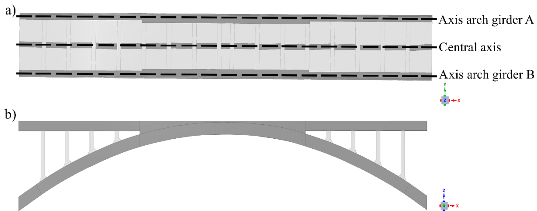
Figure 8: As-built CAD model obtained by the proposed method: a) plant view (arches A and B); and b) elevation view.
