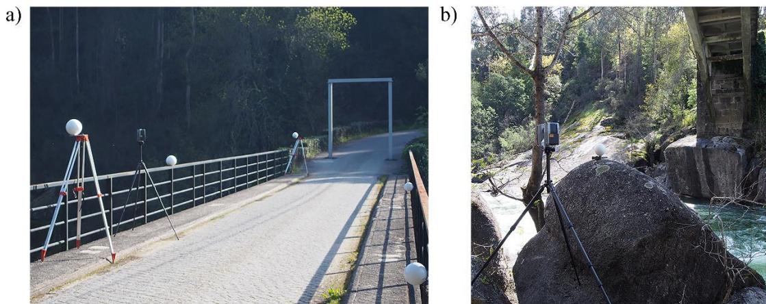
Figure 5: TLS and registration spheres used during the data acquisition: a) during the recording of the deck; and b) TLS surveying at the lower part of the bridge.
