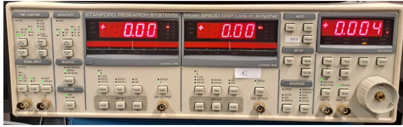
Fig. 3.3.2: Image of the lock-in SR830
