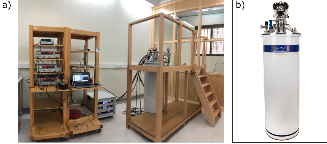
Fig. 3.5.2: a) Image of the low temperature laboratory of the university of Salamanca with a measurement equipments rack and the teslatron. b) Detail of the teslatron equipment developed by oxford instruments with a maximum magnetic field of 12 T and range of temperatures between 1.5 K to 300 K.
