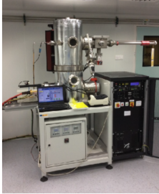
Fig. 3.2.3: e-beam evaporator designed by tecnovac with telemark e-beam gun.
