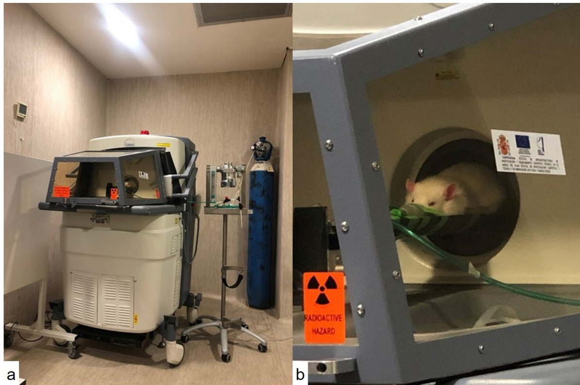
Figure 10. Radiological evaluation of the bone defect: (a) Multimodal SPECT/CT Albira II ARS scanner; (b) The study animals placed in prone position during scanning.
