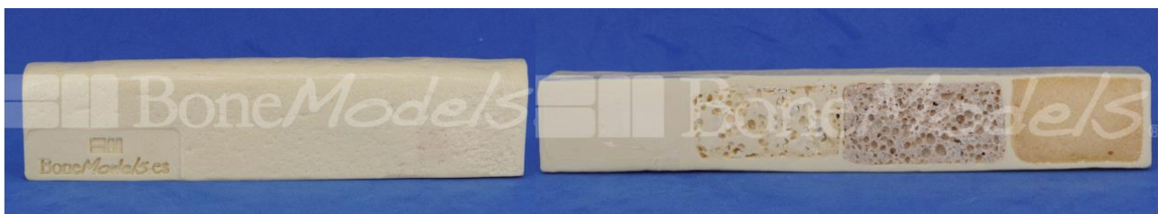
Figure 1- Artificial bone models (Bonemodels®; Castellón; Spain) with 4 types of bone densities (D1-D4).
