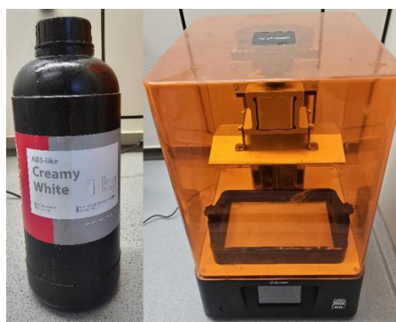
Figure 7 - 3D printer and resin material used to print the surgical guides.
