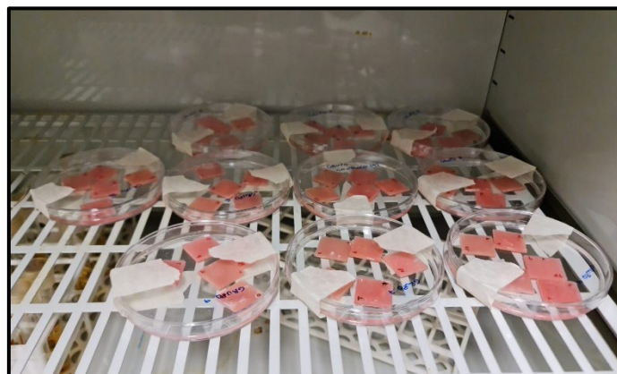
Figure 16. Specimens immersed in distilled water inside the oven
