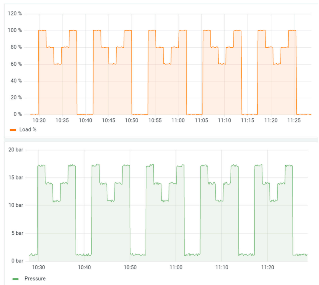
Figure 9. Dashboard through a measurement test session. The graph above represents the percentage of load with respect to the setting. The bottom graph represents the actual pressure reading of the device.
