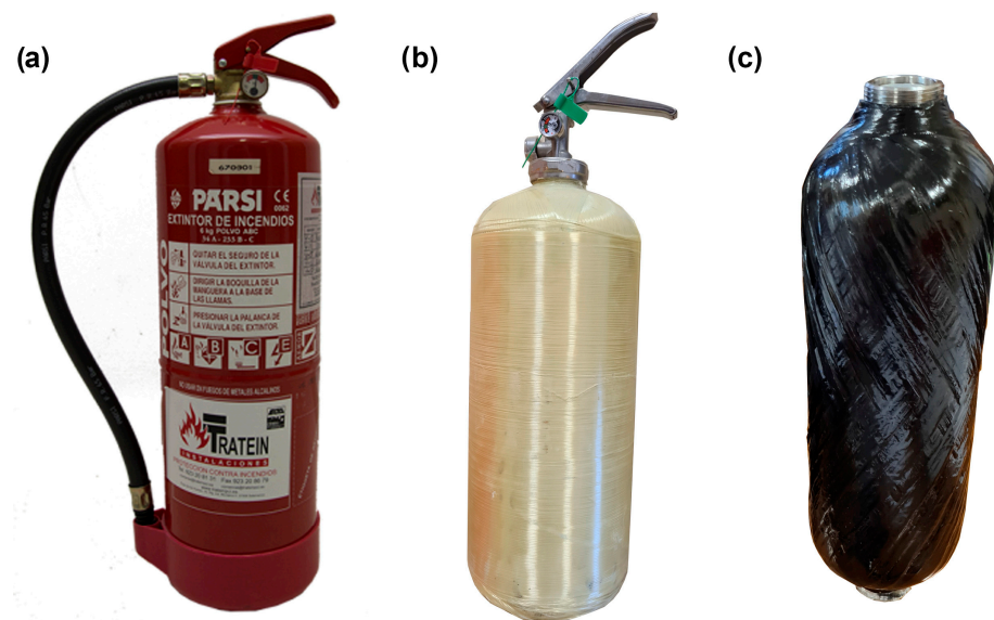
Figure 6. Vessels studied. (a) Conventional steel-based vessel; (b) AFRP-based vessel; and (c) CFRP-based vessel.
