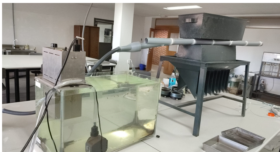
Figure 7. A sample of the experiment setup with the pipe and the water circulation pump.
