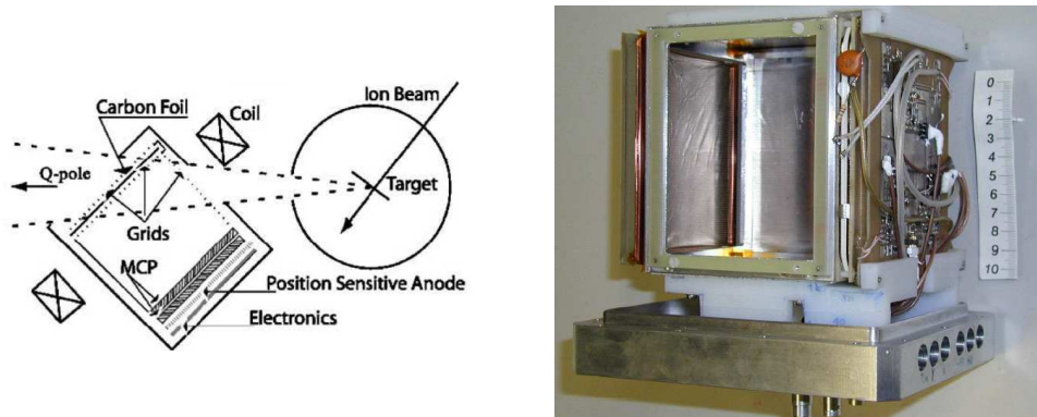
Figure 4.15: Schematic view of the setup with the reaction chamber and the MCP (left) and the MCP detector alone (right).
