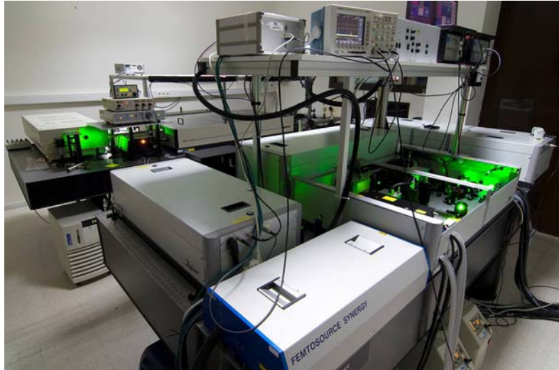
Figure 1.3. Photograph of the two CPA systems in the laboratory in Salamanca. At the front of the photo is the high-energy system (500 mJ/per pulse, Amplitude Technologies). In the back part of the photo is the Spectra-Physics system with two outputs: 1 mJ and 50 mJ/per pulse.
