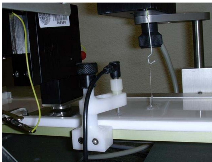
Figure III.8. Photograph of the Kelvin probe SPOT 2 model (KSV Instrument LTD) placed on the Langmuir trough.
