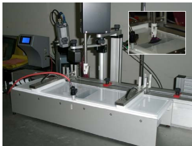
Figure III.13. Langmuir-Blodgett Standard trough (KSV Instruments). The inset shows the dipping arm which holds the substrates for the LB deposition.
