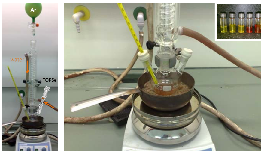
Figure V.1. Photographs of the QDs synthesis equipment set-up. The inset shows several bottles with QDs in the order that the growth of the nanocrystals occurs: from yellow (1.8 nm diameter) to red (3.4 nm diameter).
