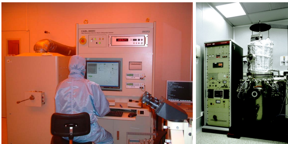
Figure III.32. Photographs of Nanolithography System for Electron Beam Lithography (CRESTEC CABL-9500C) on the left and e-beam evaporator equipment (Varian VT 118), on the right, at the Nanofabrication Clean Room in the CT-ISOM (Madrid).
