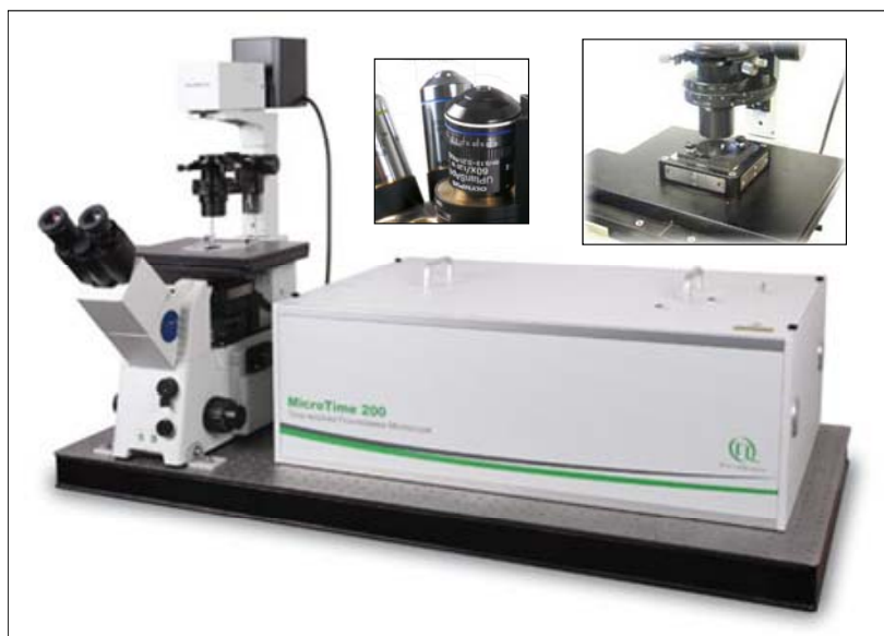
Figure III.28. External photograph of the optical unit (MicroTime 200, PicoQuant) joined to the Olympus microscope. A zoom of the objective changer (nosepiece) and sample holder is shown.
