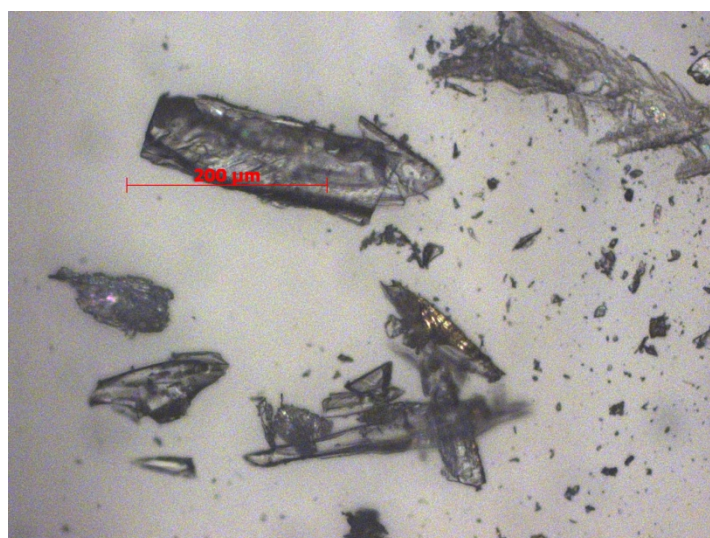
Figure IV.9. Optical microscopy image of the \text{Mg}(\text{NO}_3)_2 crystals formed on mica after the LB deposition of a polymer film prepared on saline subphase.
