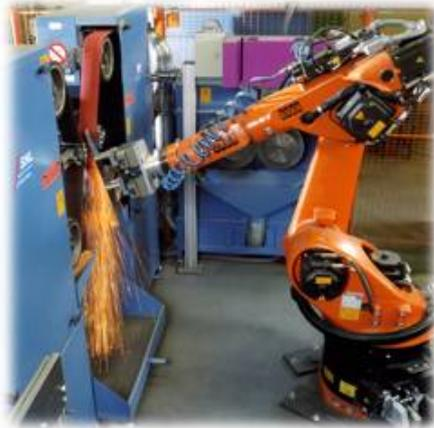
Figura 1.1: Robot KUKA KR 30 HA<sup>2</sup>.
