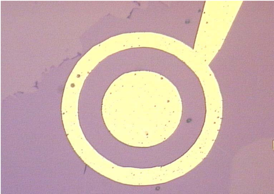
Figure 2.15 Optical image of a graphene device processed in Corbino geometry. We can see the inner and outer contacts surrounding the graphene.
