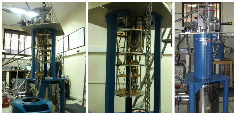
Figure 3.6 Pictures of the Triton cryostat without its radiation shields and OVC wall (left and middle). The different plates and connections can be appreciated. The picture of the right shows the cryostat successfully installed and with its tail inside the bore of the magnet (as the cryostat Heliox shown in figure 3.2).
