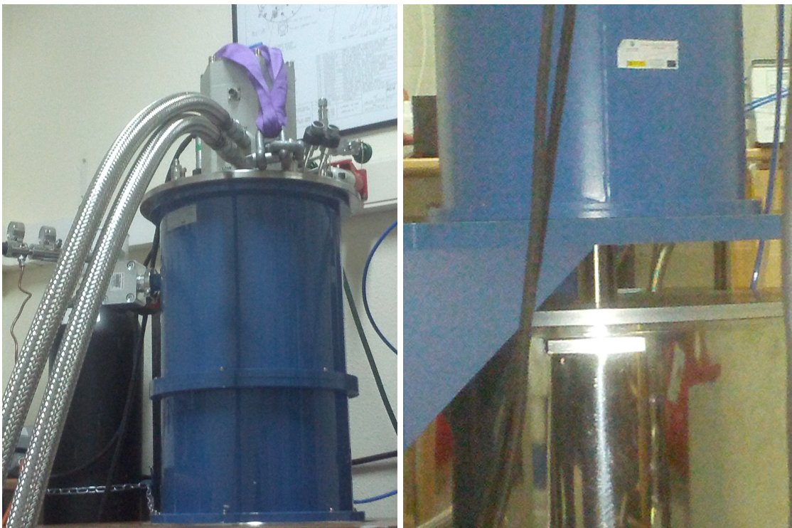
Figure 3.2 Left picture shows the top part of the cryostat with the cold head and the pulse tubes. The right picture shows the cryostat on top of the magnet. Notice that the cryostat and the magnet are physically disconnected.
