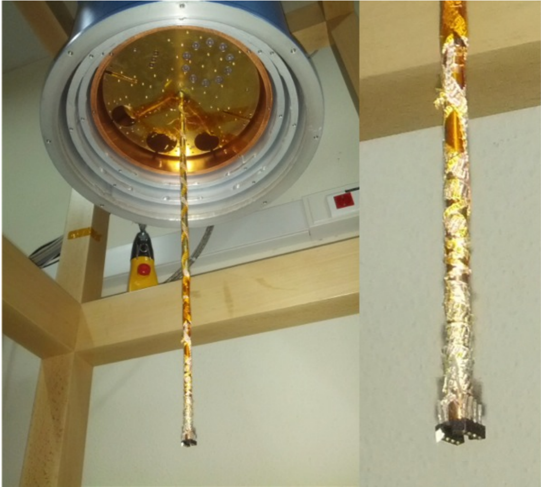
Figure 3.8 Left picture shows the whole tail from the sample holder to the mixing chamber. The right pictures shows a zoom in of the end of the sample holder and the sample holder.
