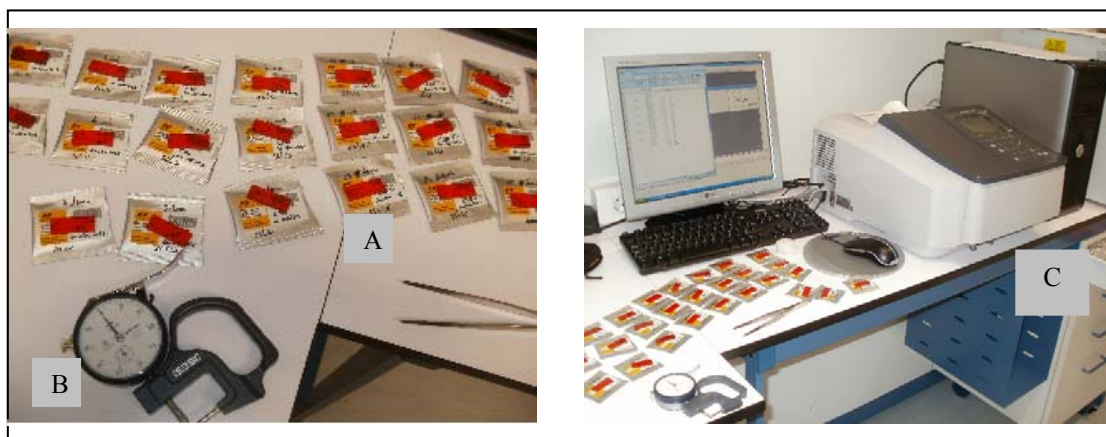
Fig. A3.6. Amber dosimeters measurement. (Dosimeters (A), Gauge for thickness measurement (B) and spectrophotometric system (C)).
