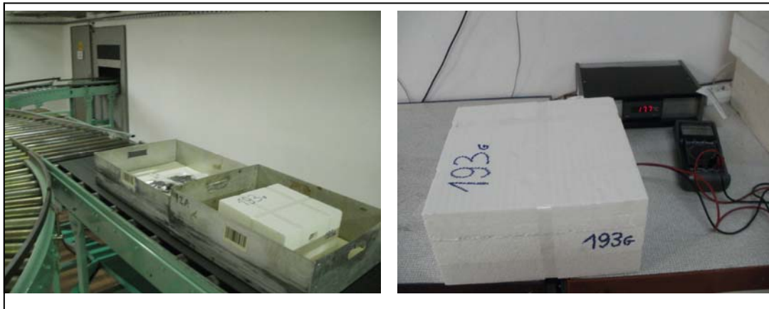
Fig. A3.10. Calorimeter in the e-beam conveyor and temperature reading.
