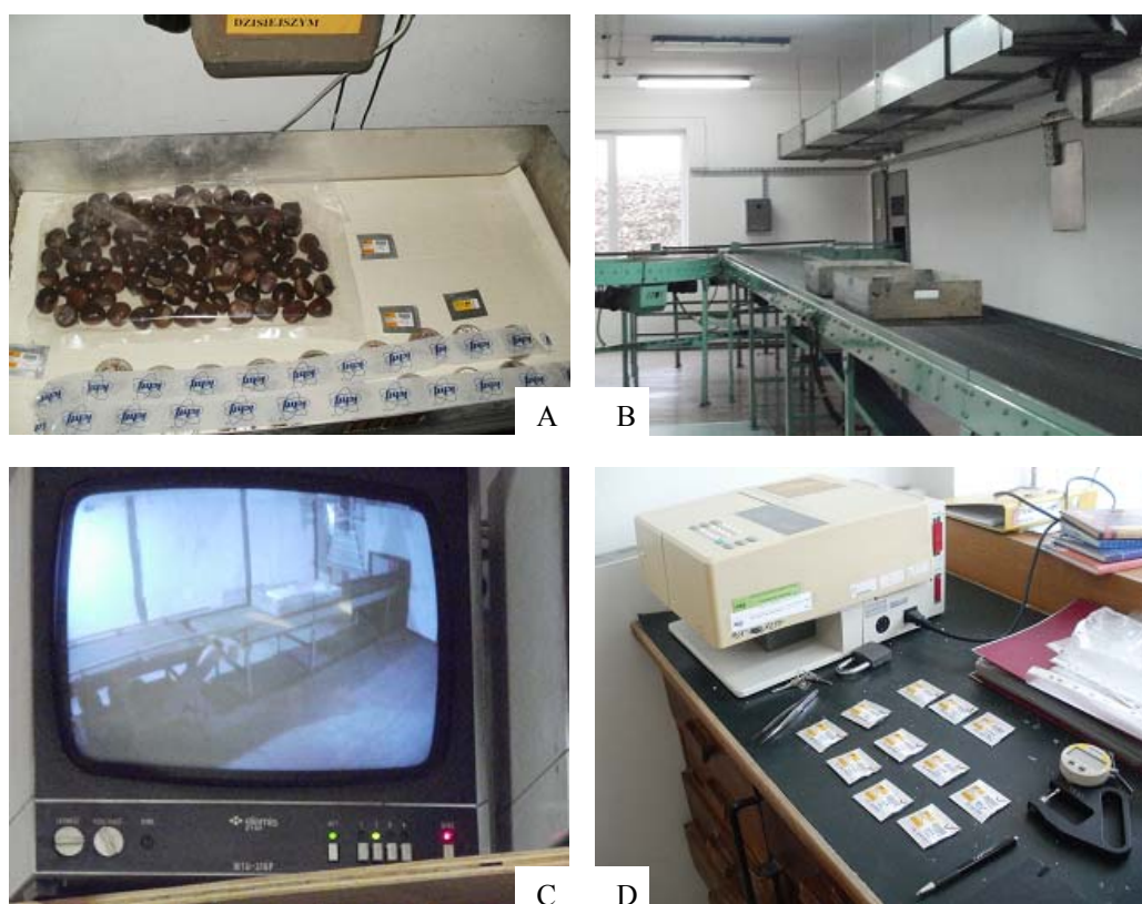
Fig. A1.13. Irradiation of chestnut fruits at INCT. (A – chestnuts in the tray, B – tray in the conveyor, C – irradiation area monitoring, D – dosimeters reading)
