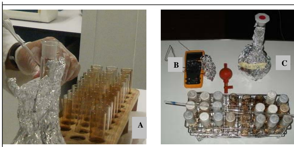
Fig. A3.4. Preparing the Fricke dosimeter. (Filling the tubes to irradiate (A); thermocouple to read solution temperature (B) and volumetric flask wrapped with aluminium foil to protect from UV's (C))
