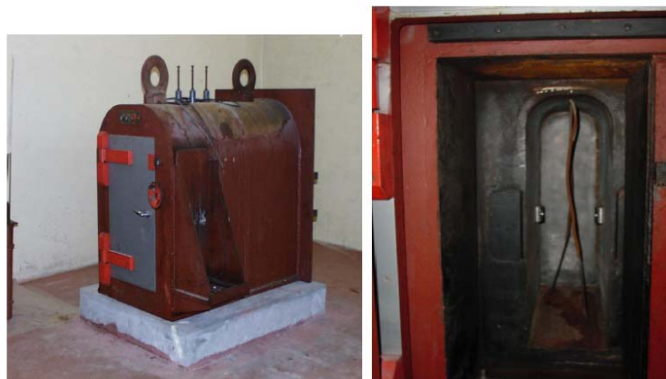
Fig. A1.1. Gamma chamber before rebuilt (outside and inside view).
