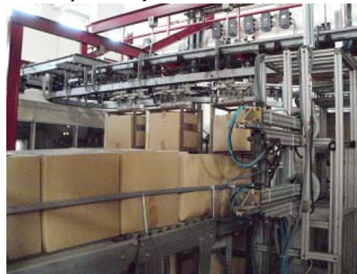
D - Pneumatic changing of boxes position.
