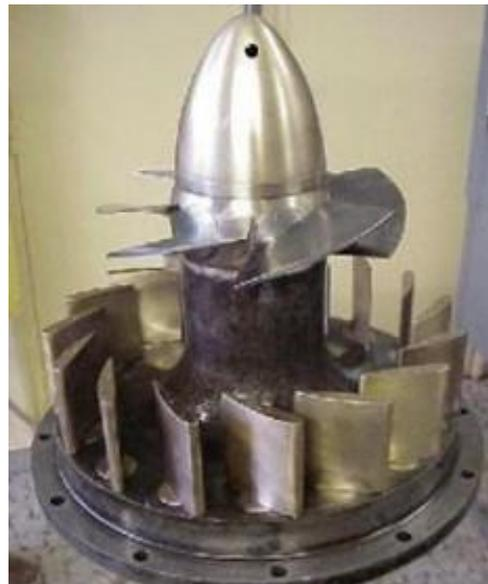
Figura 52: Turbina Kaplan (Ossberger, 2015).
