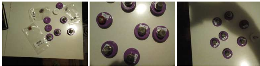
Figure 67: FM Technology: bottle stoppers serves as a socket to gas sensors
