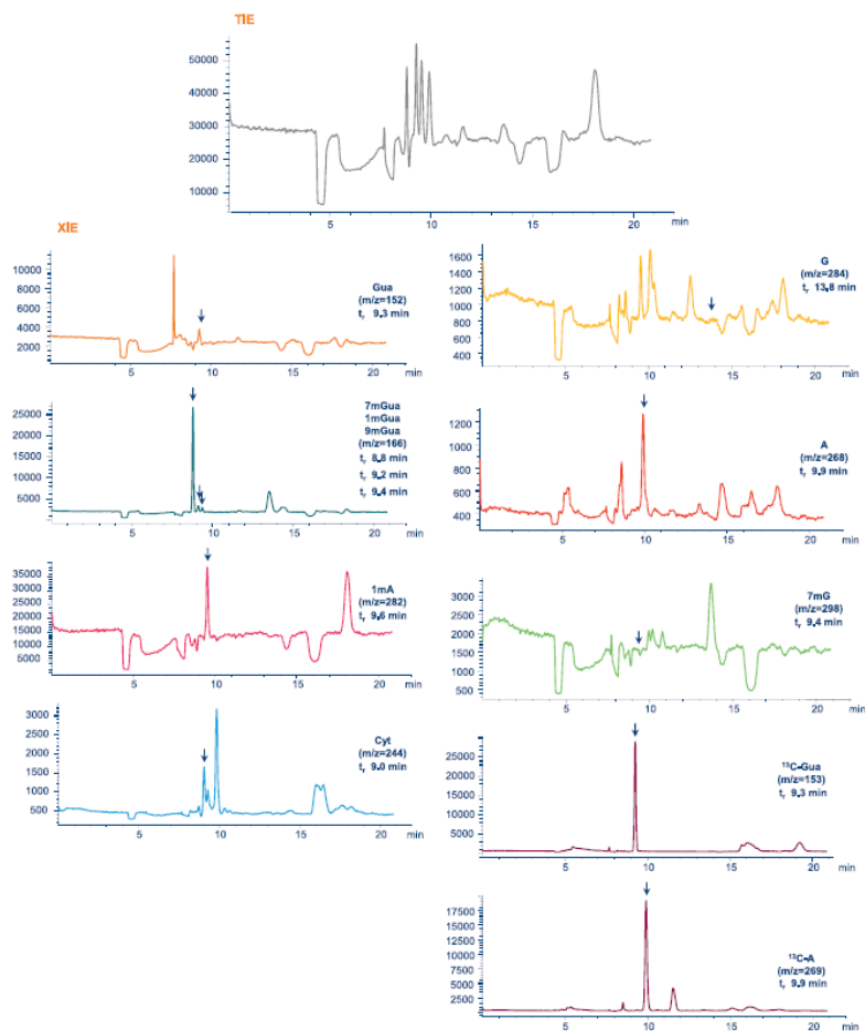
Fig. 4. Total ion electropherogram (TIE) and extracted ion electropherograms (XIE) for a urine sample directly injected in the CE-MS system. The figure includes the isotopically labeled compounds used as internal standards: ^{13}\text{C} -Gua and ^{13}\text{C} -A. The ions monitored were [\text{M} + \text{H}]^+ for all the analytes.
