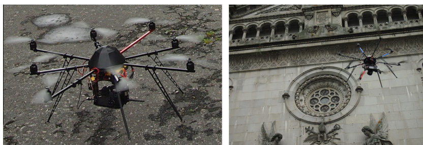
Fig. 1. Image of the UAV platform and the digital camera (left). Image taken during the data collection of the point cloud SfM (right).
