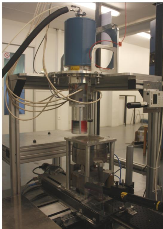
Figure 1.11: AGATA crystal in place to be scanned with the IPHC scanning system.
