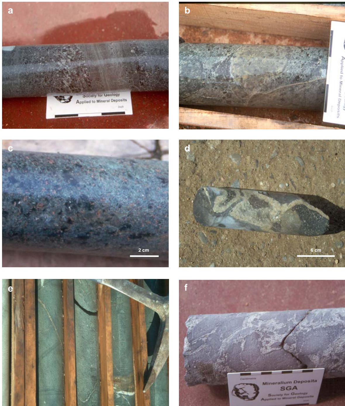
Figure 10. Photographs of the main facies of the hanging wall at Las Cruces deposit. (a) Interbedded volcaniclastic breccia, sandstone and siltstone. (b) Mass-flow deposits with clasts of dacite porphyry supported in a sand- to mud-matrix. (c) Coarse polymictic pumice sandstone composed by quartz and feldspar crystal, pumice fragments, and siltstone clasts. (d) Shale layer with pumice fragments rich in feldspar \pm quartz phenocrysts in a microcrystalline groundmass of chlorite \pm sericite. (e) Mafic sill or lava with pervasive chloritic alteration. (f) Peperite formed by interaction of felsic coherent rocks with shale.
