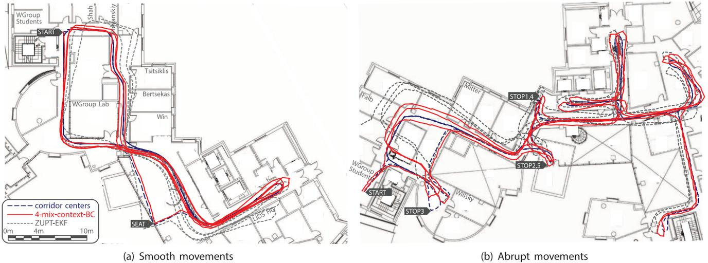
Fig. 5. The proposed context modeling avoids the rapid growth of the error over time of conventional approaches, resulting in a very high (sub-meter) accuracy. (a) Smooth movements, (b) Abrupt movements.
