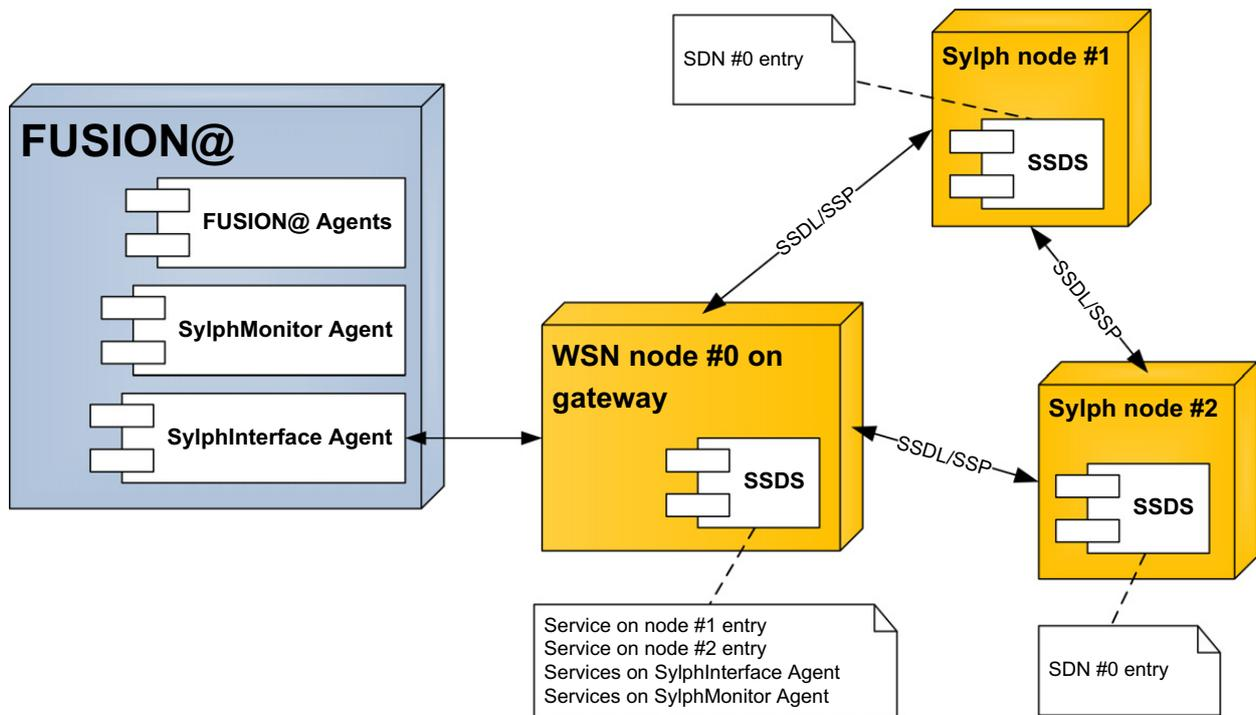
Fig. 6. UML deployment diagram of the interaction between SYLPH and FUSION@ where HERA is not yet present. Even though the features of FUSION@ provide an easy way to access SYLPH services as other services and applications, the integration of HERA into FUSION@ improves this architecture embedding agents directly on wireless sensor nodes.
