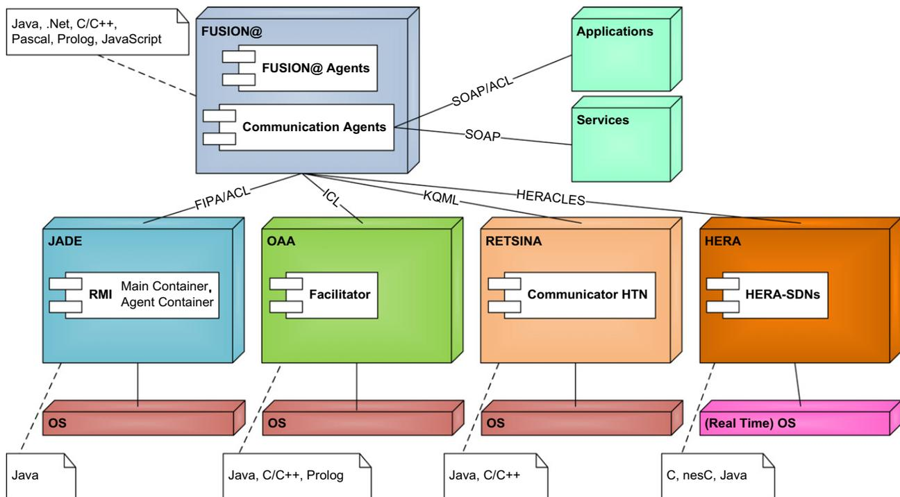
Fig. 7. UML deployment diagram representing the integration of HERA platform into FUSION@ architecture. As can be seen, HERA interact with FUSION@ as other agent platform, no matter if HERA Agents are, in fact, hardware-embedded agents running on wireless sensor nodes from different radio technologies.
