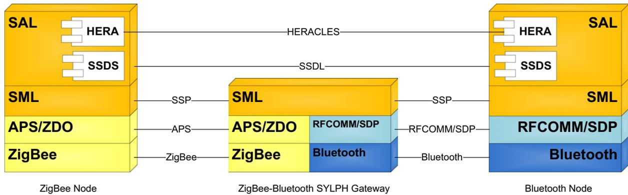
Fig. 5. UML deployment diagram of SYLPH and HERA over a ZigBee and a Bluetooth network through a SYLPH Gateway. As can be seen, HERA Agents on nodes from different radio technologies communicate each other in a transparent way thanks to SYLPH.
