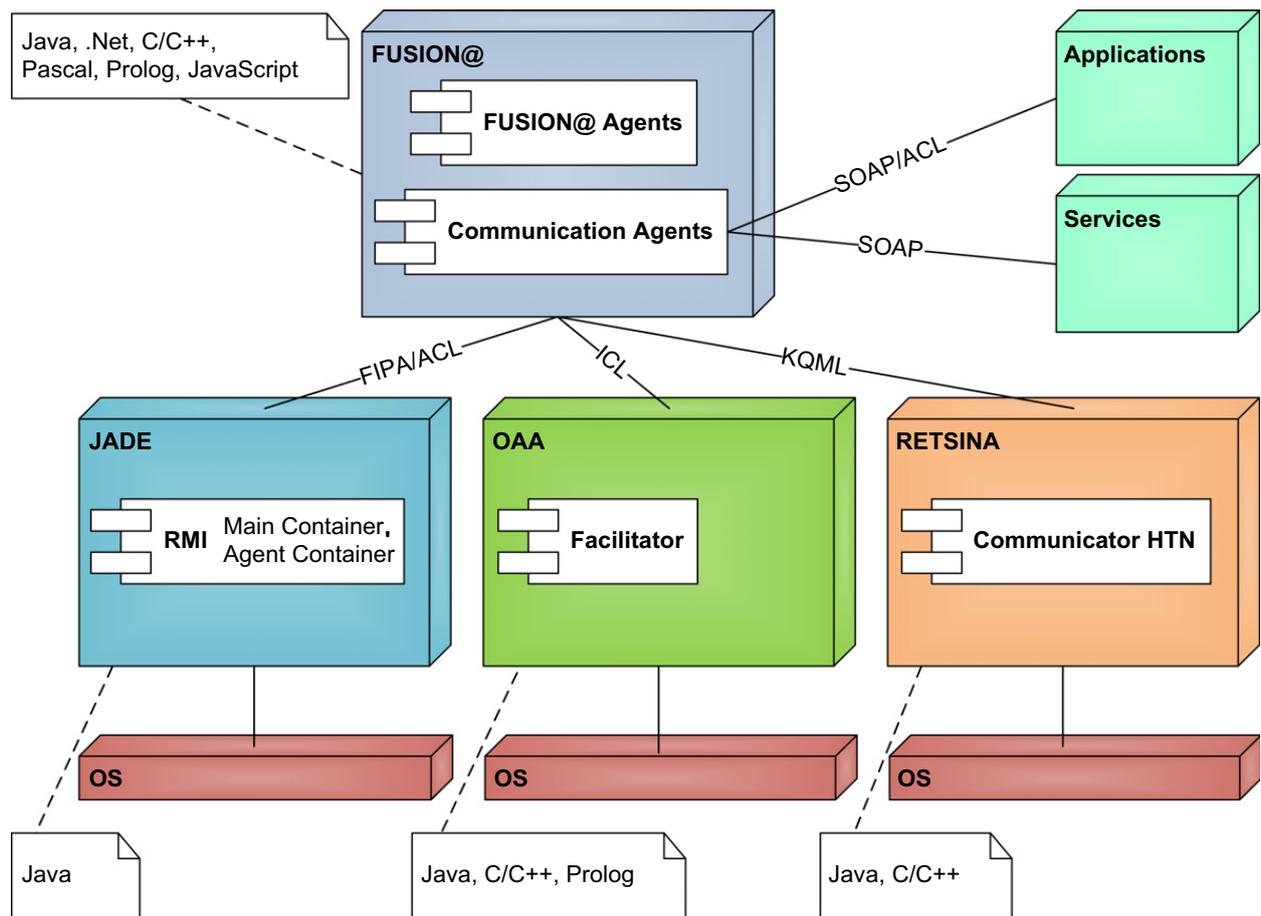
Fig. 1. UML deployment diagram of the basic schema of the FUSION@ architecture. The association between FUSION@ and each agent platform is defined according to its respective communication protocol. In a similar way, communication protocols are also used to associate the FUSION@ architecture itself with both services and applications.
