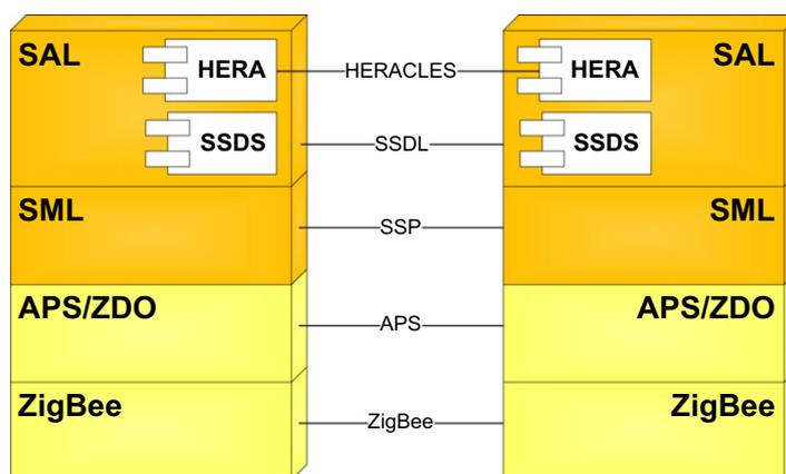
**Fig. 2.** UML deployment diagram of the HERA platform running over SYLPH. This diagram shows the HERA Agents layer running as a component on the SYLPH Application Layer. Likewise, it can be seen the different layers of SYLPH and HERA, as well as the different protocols that communicate each layer on different ZigBee nodes.
