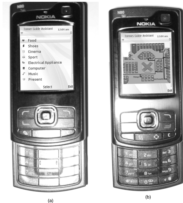
Figure 7. Screenshot representing how a client indicates his preferences (a) and the plan suggested to the client (b)
