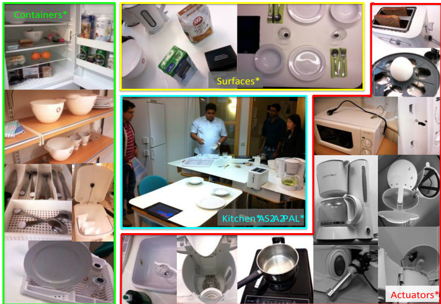
Fig. 2. Network of RFID readers and simple state change sensors embedded in containers, surfaces and actuators forming the sensing backbone of the Kitchen AS-A-PAL
