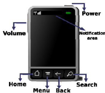
Fig. 2. Structural elements of a smartphone that could hinder its use
