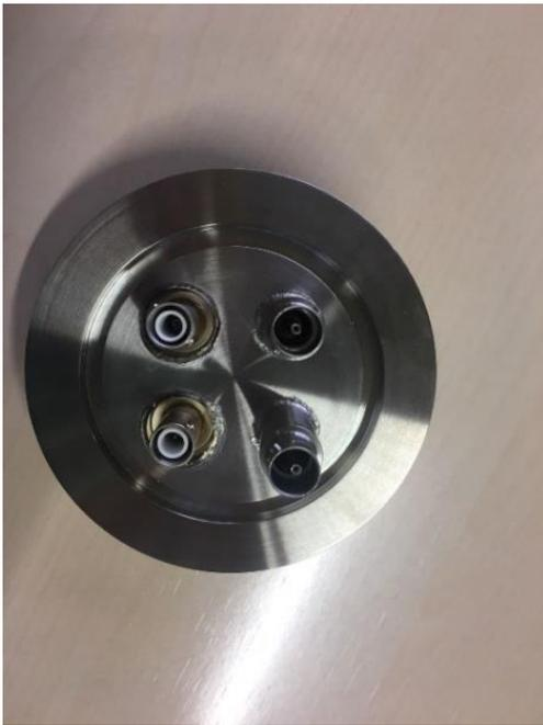
Figura 169. Feedthrough vista frontal.
