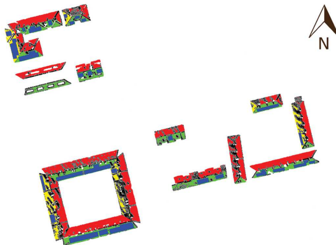
Figure 11. Georeferenced point cloud of the detail zones after the process. Optimal surfaces (rectangles) for the installation of solar panels are highlighted in blue. Roof ID's are used in Table 4.
