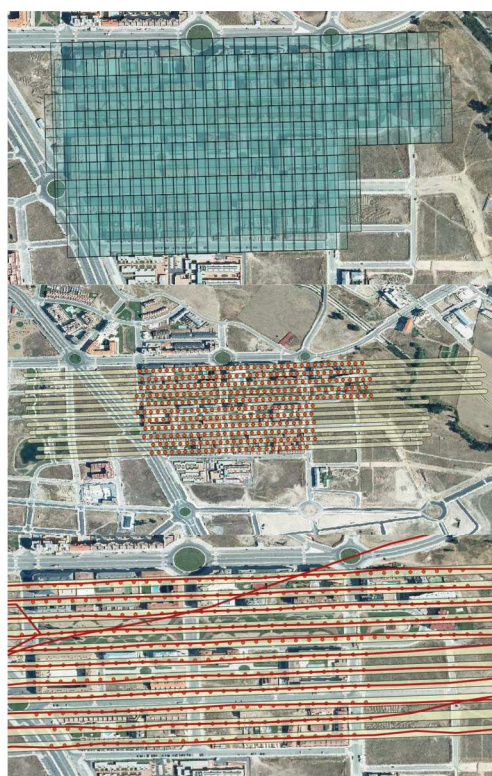
Figure 6. Flight planning: (Top) Areas captured by each image shot for the thermographic sensor. (Middle) Flight planning for the navigation of the aerial trike. (Bottom) GPS track after the aerial trike flight with the position of each image shot.
