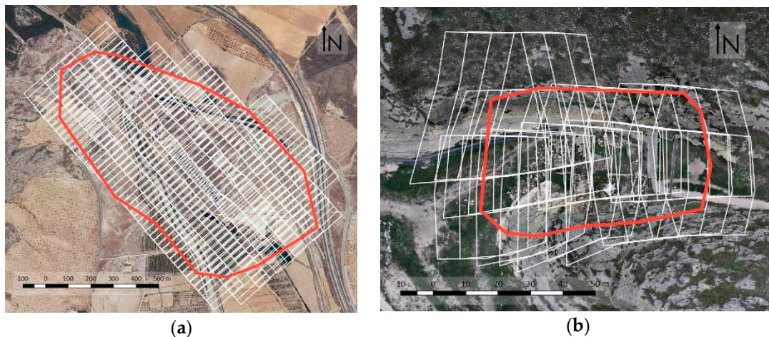
Figure 3. Example of image footprints projected over terrain (white line) and the different workspaces (red line). (a) Paratrike flight planned over the whole area and (b) UAV flight planned over “El Reguerón” area.
