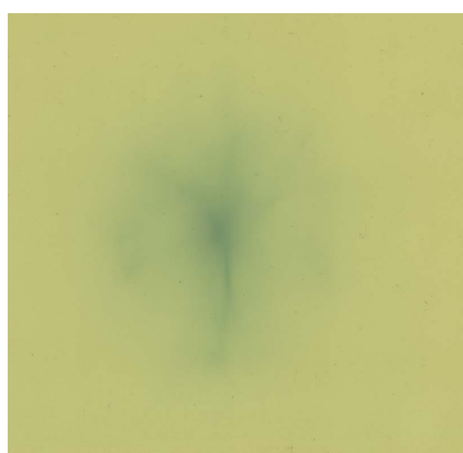
Figure 6.11: Scanned image of a RCF after being developed by five consecutive laser shots.
