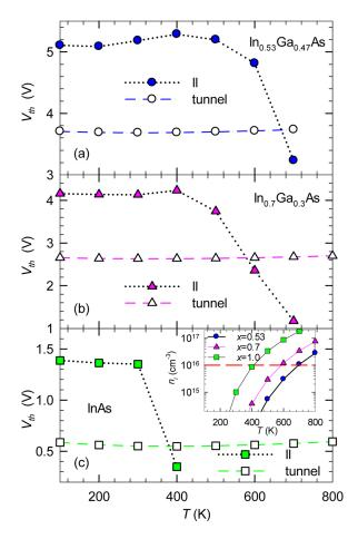
FIG. 3. MC values of  $V_{th_{1}II}$  and  $V_{th_{1}III}$  as a function of T for (a)  $In_{0.53}Ga_{0.47}As$ , (b)  $In_{0.7}Ga_{0.3}As$ , and (c) InAs 100 nm PIN diodes. Inset of Fig. 3(c):  $n_i$  as a function of T for the three materials.
