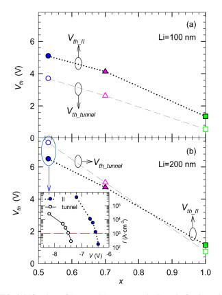
FIG. 2. MC values of  $V_{th \ II}$  and  $V_{th \ tunnel}$  vs. the In mole fraction x in In<sub>x</sub>Ga<sub>1-x</sub>As (a) 100 nm and (b) 200 nm PIN diodes at room temperature. Inset: MC values of the I–V curves when considering exclusively II processes or band-to-band tunneling in the simulations of an In<sub>0.53</sub>Ga<sub>0.47</sub>As 200 nm PIN diode at room temperature.
