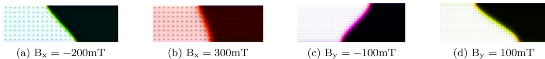
Fig. 5. Snapshots of different shapes of the DWs observed under a current density of J_x = 0.1 \text{ TA/m}^2 in Pt/CoFe/MgO after 5 ns. (a) and (b) show a rigidly moving linear DW, while the DW in (c) and (d) is rather S-shaped.
