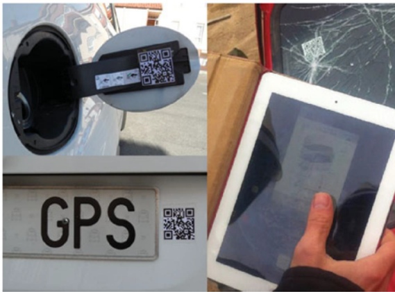
Figure 3. Strategic QR codes' location in the vehicle: door of the fuel tank (top left), top corner of the windscreen (right) and next to the rear plate (bottom left).
