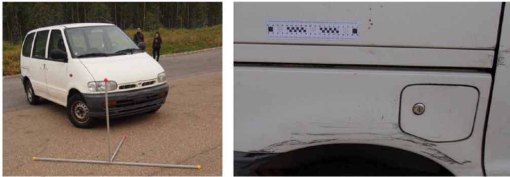
Figure 1. (Left) Metallic scale bar used in the general point cloud. (Right) Magnetized targets used for obtaining the deformation map (detailed point cloud). The metallic scale bar features four branches, each 1 m long from the center point. The magnetized target is 20 cm long.
