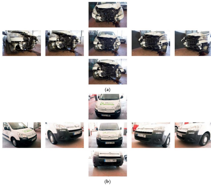
Figure 6. Data acquisition protocol used to digitalise the car’s frontal: (a) deformed model; and (b) non-deformed model.
