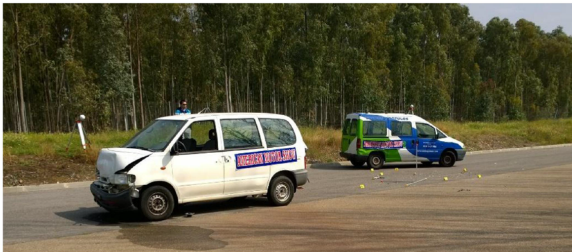
Figure 4. Final position of the crashed vehicles involved in the simulated accident. It can be appreciated (between both cars) the metallic scale bar used for providing metric capabilities to the photogrammetric reconstruction.
