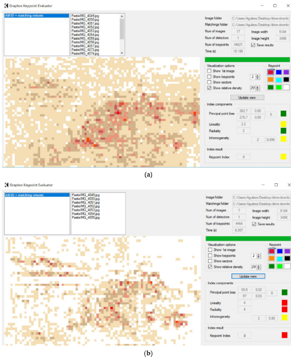
Figure 8. Results obtained during the analysis of the distribution of the key points extracted along the camera’s sensor: (a) AMSD, robust matching, and camera’s sensor spatial filtering; and (b) AMSD and robust matching without camera sensor’s spatial filtering.
