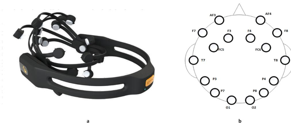
**Figure 21 ECG interface. a) EPOC+ helmet of Emotiv b) Distribution of EPOC+ helmet sensors in the head of subjects**
