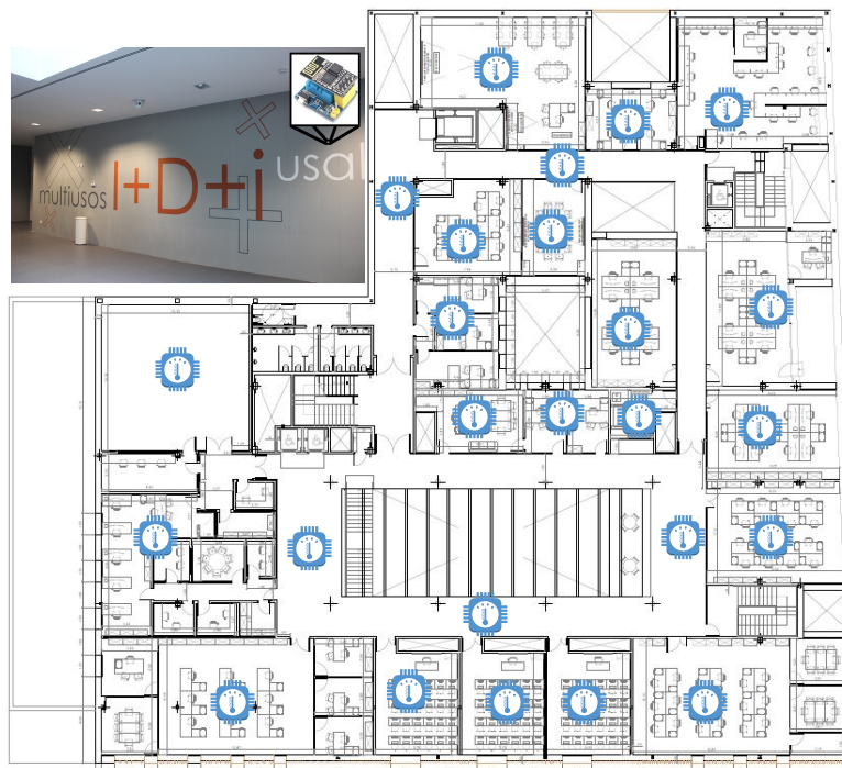
FIG. 5.1: Map of the building with all the sensor placed, a sample of an indoor surface for testing our model and a sample of a sensor.
