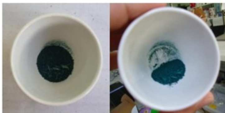
Figure III.12: Kaolinite functionalized with aluminum(III) tetranitrometallophthalocyanine.
