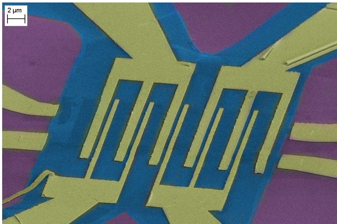
Figure 4.25 False color tilted SEM image of an ADGG-GFET which has a finger bent and a delamination problem.
