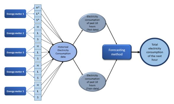
Figure 1: Perspective of the data sources and data collection \*H: Air conditioning systems, L: Lights, S: Sockets
