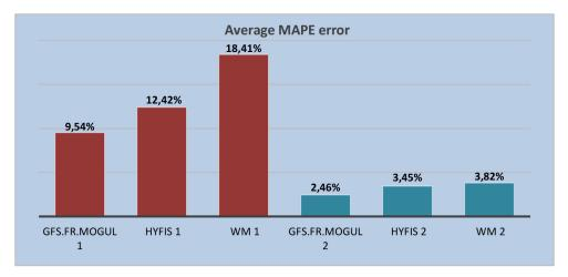
Figure 3 - Figure 4: Average MAPE errors of the forecasted electricity consumption values of TRT building and N building
