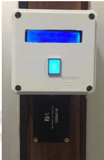
Figure 1. Access control system
