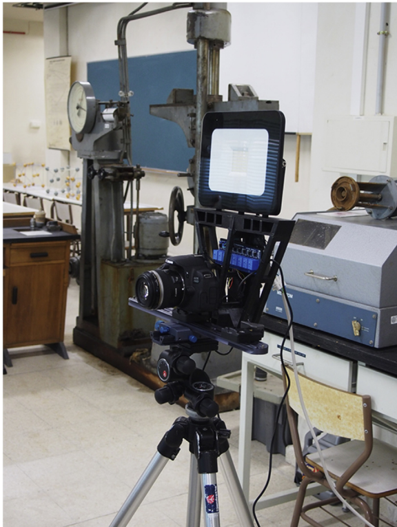
Fig. 4 – Experimental prototype used during the traction tests in the specimens.
