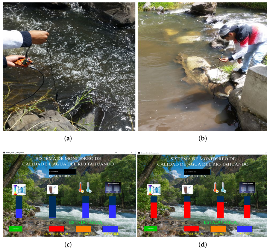
Figure 10. System testing and visual interface. (a) Testing embedded system developed in the rural sector. (b) Testing embedded system developed in urban sector. (c) Visual interface showing low level of contamination. (d) Visual interface showing high level of contamination.
