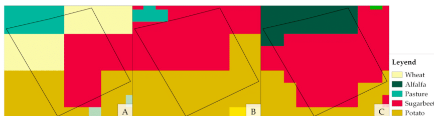
Fig. 8. Pixel-based crop classification for the 210th plot of the field visits performed by the Duero basin fluvial guards in 2017 summer period from the quickest to the slowest classifier. (a) Using Decision Trees (DT). (b) Using Weighted Nearest Neighbor (WNN). (c) Using Ensemble Bagged Trees (EBT).
