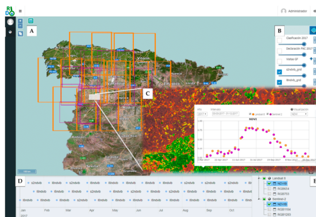
Figure 6. Screenshot of the web-GIS module. (A) web-GIS viewer; (B) Several layers to visualize, i.e. S2 and L8 grids, 2017 crop classification (source: Agrarian Technological Institute of Castilla y León, ITACYL), crop declarations to the Common Agricultural Policy (CAP) and field inspections; (C) Usual NDVI variation graphic for an irrigated summer crop: user could choose to visualize NDVI values from L8, S2 or both satellite platforms; (D) Timeline and images availability depending on the area shown by the viewer; (E) Selection of derived products to visualize: RGB (Red, Green and Blue) false colour and NDVI images from both L8 and S2.
