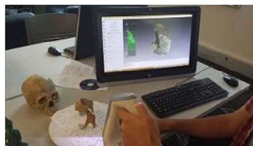
Fig. 3 Digitization of bone pieces with Artec Eva model hand scanner and graphic workstation
