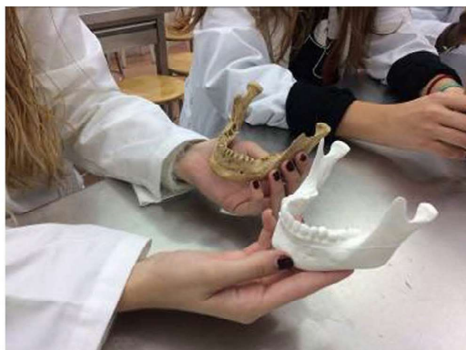
Fig. 10 3D model of the jaw printed with polylactic acid (PLA), compared with a real piece
