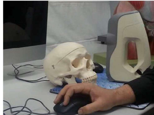
Fig. 2 Hand scanner model Artec Eva used for the digitalization of bone pieces
