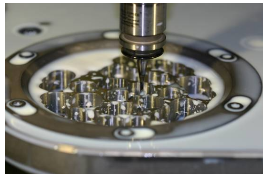
Fig. 4 Milling of cobalt-chromium specimens
