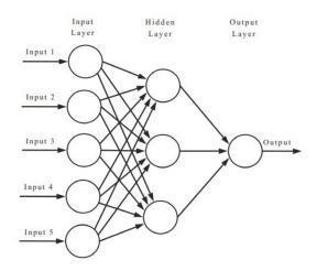
Fig.2. Artificial Neural Network Architecture.
