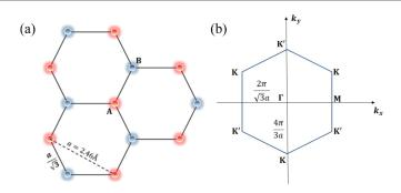
**Figure 1.** Scheme of graphene's structure in (a) direct and (b) reciprocal space. The unit cell is composed by two carbon atoms (red and blue). In the reciprocal space, points K and K' correspond to the location of the Dirac cones. In our study the laser pulse is linearly polarized along the y direction and it is aimed perpendicularly to the graphene layer (x–y plane).
