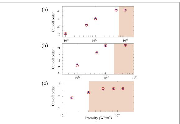
**Figure 3.** Cut-off scalings with intensity for a 8 cycle pulse with wavelengths (a) 3  $\mu$ m, (b) 1.6  $\mu$ m and (c) 800 nm. The blue diamonds correspond to the numerical integration of the TDSE. The red circles are given by the semiclassical model SPAM (more details are given in the text). Filled areas correspond to intensities above damage threshold.
