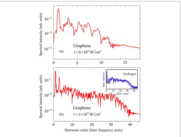
**Figure 2.** HHG spectra from SLG driven by a 3  $\mu$ m wavelength, 28 fs (2.9 cycles) FWHM pulse at two different intensities: (a)  $5 \times 10^{10}$  W cm<sup>-2</sup> and (b)  $1 \times 10^{12}$  W cm<sup>-2</sup>. As a reference, the inset shows the HHG spectrum emitted by the hydrogen atom, driven by a 800 nm pulse with the same number of cycles, at an intensity of 1.57  $\times 10^{14}$  W cm<sup>-2</sup>.
